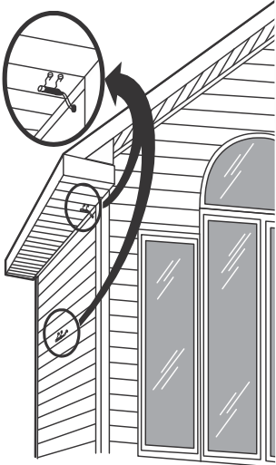
Fig. 25. Typical locations for OAS-1 Outdoor Sensor.
