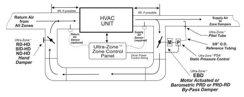
*Note:* This EWC Controls drawing of the Bypass damper, Hand Damper, Static Pressure control and Related duct-work is intended to serve only as a guide. Your actual duct-work layout and components may differ. Use the graphic as a guide when planning or designing a Zone system regardless of the Equipment type, Duct layout and Airflow configuration.
