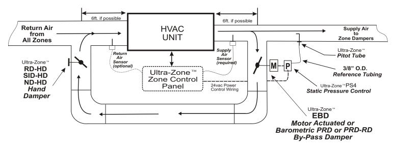
*Note:* This EWC Controls drawing of the Bypass damper, Hand Damper, Static Pressure control and Related duct-work is intended to serve only as a guide. Your actual duct-work layout and components may differ. Use the graphic as a guide when planning or designing a Zone system regardless of the Equipment type, Duct layout and Airflow configuration.
