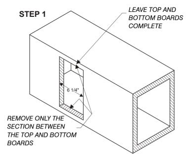
Each kit should contain two identical side brackets. Remove a section of the duct 6 1/4" wide. Cut between the top and bottom boards being sure to leave them in place, including their edge.
