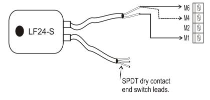
NOTE: LF24 does not have end switch or second pig tail.
