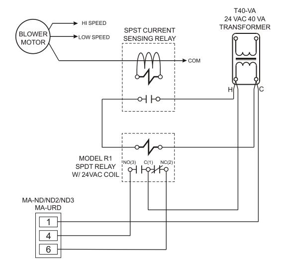
\*DAMPER WILL OPEN TO BRING IN FRESH AIR / COMBUSTION AIR WHENEVER BLOWER ENERGIZES
