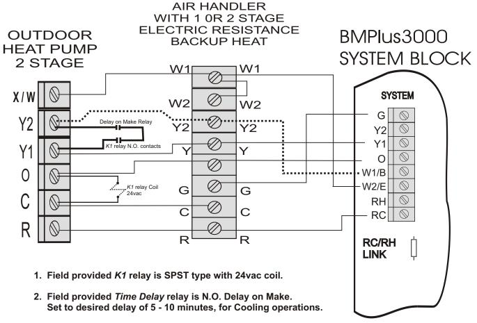
3. Connection from W1/B to Y2 results in immediate 2 stage Heating Operations.
