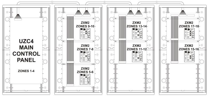
DO NOT CONNECT OR DISCONNECT BUS CABLES WHILE POWER IS APPLIED TO THE SYSTEM. DOING SO <u>MAY DAMAGE</u> THE ZXM2 MODULES AND VOIDS ALL WARRANTIES.
