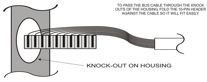
FIELD BUS CABLES ARE ROUGHLY 40" IN LENGTH, SECURE CABLE AS NECESSARY.
