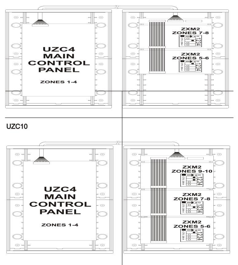
DO NOT CONNECT OR DISCONNECT BUS CABLES WHILE POWER IS APPLIED TO THE SYSTEM. DOING SO <u>MAY DAMAGE</u> THE ZXM2 MODULES AND VOIDS ALL WARRANTIES.
