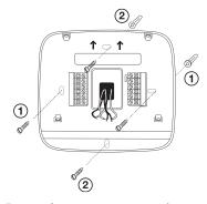
For vertical mount put one screw on the top and one screw on the bottom. For horizontal mount put one screw on the
