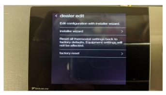
**Step 1:** Using the Daikin ONE+ thermostat connected to Zone 1 only, navigate to "**Dealer Edit**", insert the password and select the *Installer Wizard*.
