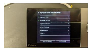
Step 5: Select "System Test" to advance to the next screen. You can navigate back to this screen after the system test is complete, and select "Charge Mode" to confirm that the refrigerant level in your system is correct.
